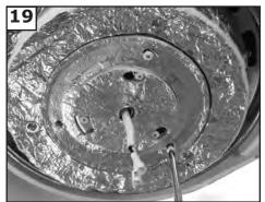
Loosen 2 screws and remove 1 screw from light plate and save screw.
